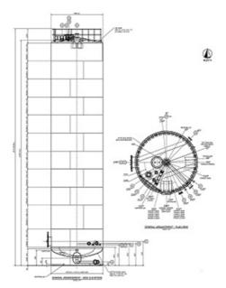
All elements of design considered Australian and International standards to optimise the life and performance of each tank. Structural design considered the density of stored fuels - diesel and ULP, along with the venting requirements for petrochemicals, in accordance with AS1692. Additional components were added to each tank; these included access points for maintenance and internal floating roof systems to create vapour barriers.
